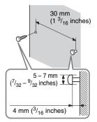
**3** Hang the IR transmitter via hole on the bottom of the stand on the screw.
