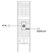
1 Press "DISPLAY when the system is in stop mode.
