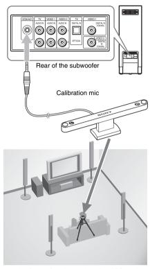
The front of each speaker should face the calibration mic, and there should be no obstruction between the speakers and the calibration mic.
