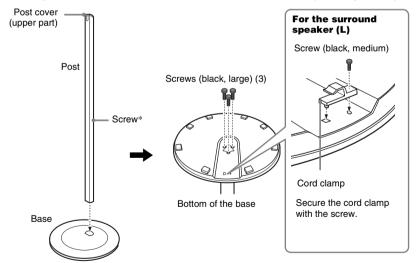
\* Do not remove the screw that is attached to the post. The screw is to prevent the speaker from slipping.
