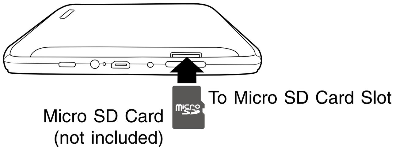
Insert the micro SD card, with contacts facing the screen, into the tablet's Micro SD slot until it clicks.
