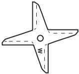
**Wet-Blade Container:** Designed for processing liquids, including juice, frozen mixtures, sauces, soup, purees, batter, and for wet chopping. The wet blades can also process grain and knead dough, but they are not quite as efficient as the dry blades in this application. See instructions for dry container use.
