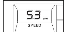
Each time a button is pressed, the speed setting will change by 0.1 mph; if a button is held down, the speed setting will change in increments of 0.5 mph. To change the speed setting quickly, press one of the twelve Quick Speed buttons. **Note: The console can display speed and distance in either miles or kilometers (see THE SPEED DISPLAY on page 14). For simplicity, all instructions in this section refer to miles.**
