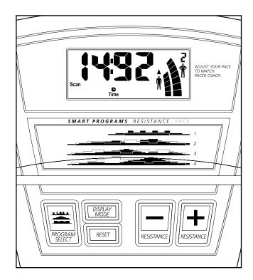
The advanced console offers a selection of features designed to make your workouts more enjoyable and effective. When the manual mode of the console is selected, the resistance of the pedals can be adjusted with a touch of a button. As you exercise, the console will provide continuous exercise feedback. You can even measure your heart rate using the built-in hand-grip pulse sensor. (For information about an optional chest pulse sensor, see page 11.)
