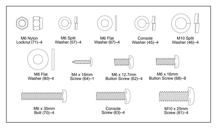
Attach the Stabilizer (8) to the Frame (1) with four M10 x 25mm Screws (81) and four M10 Split Washers (46).
