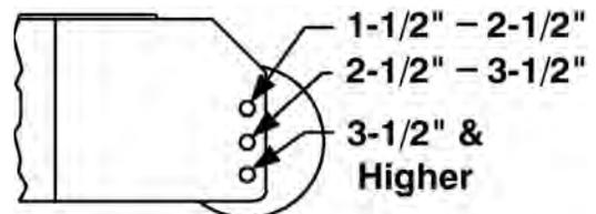
Height of cut ranges for roller adjustment
