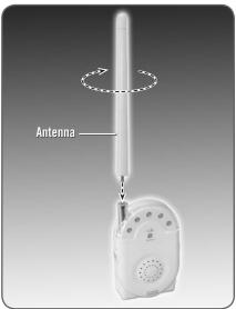
• Fit each antenna into the socket in the receiver and the transmitter. Turn the antennas to secure in place. **IMPORTANT!** This product is designed to operate properly with the antennas provided. To reduce the chance of potential radio interference to other users, assemble and use only the antennas provided.
