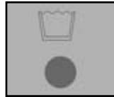
**WATER FULL :** A warning signal (beep) will sound and the adjacent red indicator light will **flash** continuously indicating the *internal reservoir* is full. See "Internal Safety Feature" on pg.5 for additional details.
