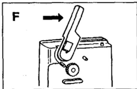
Push can opener lever to the right to remove it from the recessed area (F).
