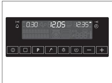
When the time has elapsed, an audible signal sounds for 2 minutes. The oven switches itself off. "0.00" and the End Time arrow
