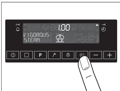
5. Stop the signal and switch off the oven by pressing the main power switch
