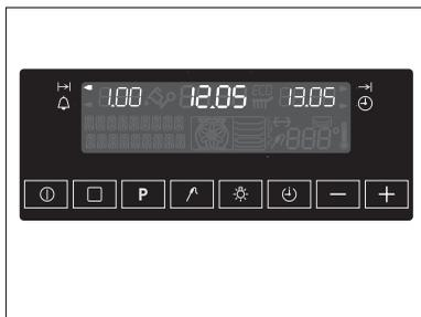
When the time has elapsed, an audible signal sounds for 2 minutes. The oven switches itself off. "0.00" and the Cooktime arrow
