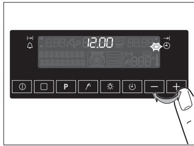
3. After about 5 seconds, the arrow stops flashing and the clock displays the time set. The appliance is now ready to use again.
