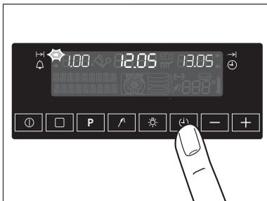
3. Using the END TIME
