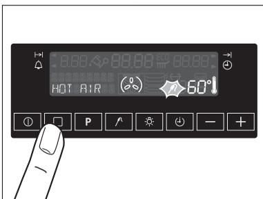
4. Start setting the desired core temperature within 5 seconds, using the
