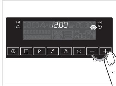
The flashing stops and the clock displays the time of day set.
