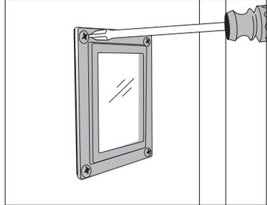
5. Re-fit metal frame and seal and tighten screws.
