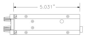
ALLOW UP TO 2.500" FOR REAR CONNECTOR AND CABLE CLEARANCE
