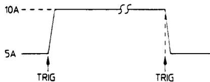
**Figure 2-7. Toggled Transient Operation**
