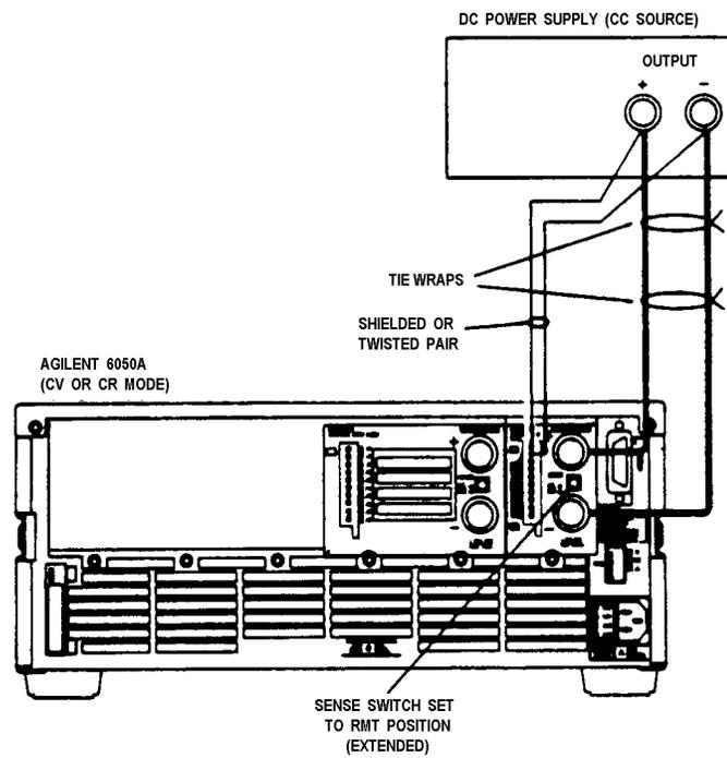
Figure 3-13. Remote Sensing
