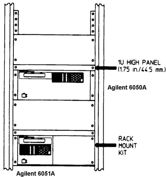
Figure 3-4. Rack Installation
