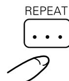
To repeatedly play the displayed track, press the **REPEAT button** once. The REPEAT-1 indicator lights. The **REPEAT button** can be pressed in any playback mode.
