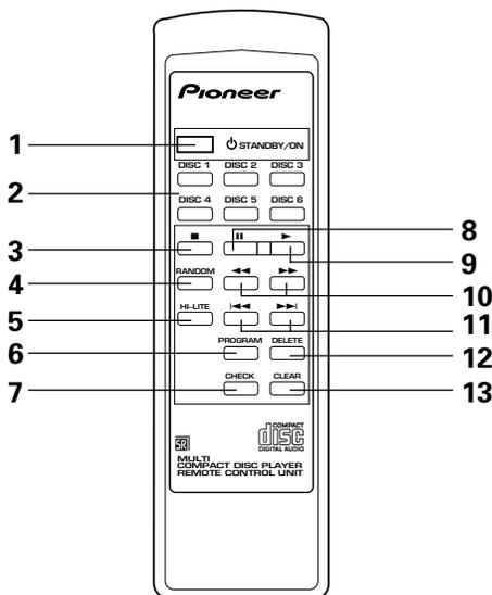
Remote control buttons with the same names or marks as buttons on the front panel of the player control the same operations as the corresponding front panel buttons.
