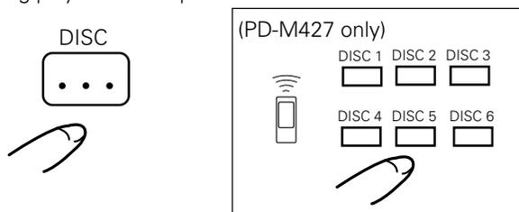
Use the **DISC button** to select the desired disc number, then press the **▶/II button**, or one of the **DISC NUMBER (DISC 1-DISC 6) buttons**; the player will then search for the selected disc and begin playback from the beginning of the disc.
