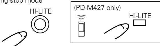
When the **HI-LITE button** is pressed once during stop mode, playback starts from a point 1 minute after the beginning of the first track, and the first track of each disc is played for about 10 seconds. The DISC SCAN indicator blinks during Disc Scan mode. After the first tracks of all discs are scanned, the player enters stop mode.
