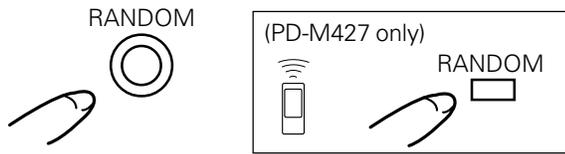
Press the **RANDOM button**. All tracks on all discs are played in a random order. To play tracks other than the deleted tracks in a random order, press the **RANDOM button** after carrying out the Delete Program procedure. See "Delete Program Playback" on page 13.
