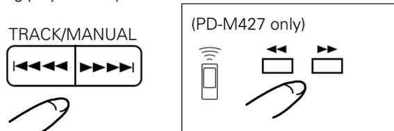
While the **▶▶▶▶ button** is kept pressed, playback rapidly advances toward the end of the disc. When playback reaches the end of the disc, the player enters pause mode and “END” is displayed. While the **◀◀◀◀ button** is kept pressed, playback rapidly reverses toward the beginning of the disc. When the desired passage is reached, release the **▶▶▶▶ button** or **◀◀◀◀ button**. The player enters original mode (playback or pause) where **▶▶▶▶ button** or **◀◀◀◀ button** is released.
