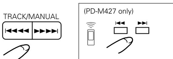
When the **▶▶▶▶ button** is pressed once or a number of times, playback advances to the beginning of a track located after the track being played. The position of the located track corresponds to the number of times the button is pressed. When the **◀◀◀◀ button** is pressed once, playback returns to the beginning of the track being played. When this button is pressed more than once, playback is returned to a track located before the track being played.
