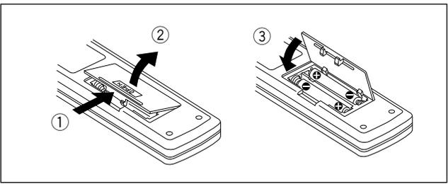
Open the lid of the battery compartment on the rear of the remote control unit, and insert the batteries (size "AAA" (IEC R03)), taking care to align the ⊕ and ⊖ polarities correctly.
