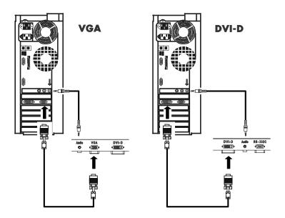
You may connect the TV to a PC or other equipment with a VGA cable or a digital interface compliant with the Digital Visual Interface (DVI) standard. Use a DVI-D 29-pin signal cable when making connections to the DVI connector. This connector supports HDCP, a form of copy protection. Note that the DVI terminal does not support analog RGB input.
