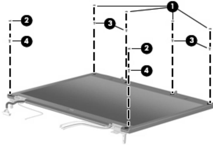
8. Flex the inside edges of the left and right sides (1) and the top and bottom sides (2) of the display bezel until the bezel disengages from the display enclosure.
