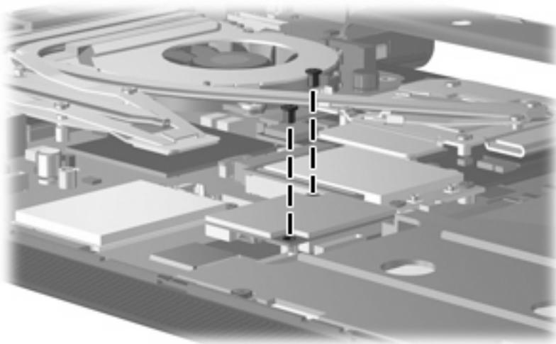
**Where used:** 2 screws that secure the modem module to the system board
