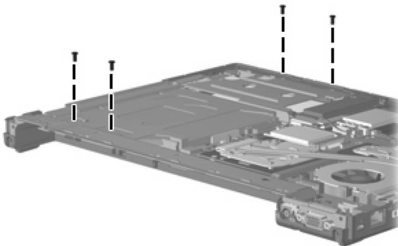
**Where used:** 4 screws that secure the system board frame to the base enclosure
