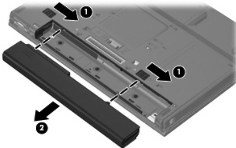
Install the battery by inserting it into the battery bay until you hear a click.
