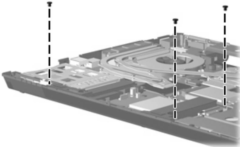
**Where used:** 3 screws that secure the speaker assembly to the base enclosure
