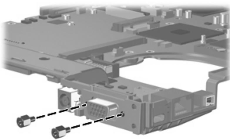
**Where used:** 2 screw locks that secure the system board to the system board frame
