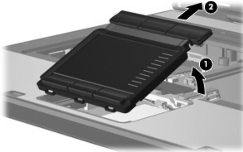
6. Disconnect the TouchPad cable **(1)** from the system board.
