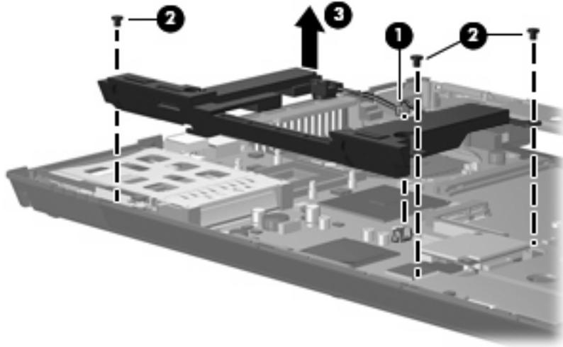
Reverse this procedure to install the speaker assembly.
