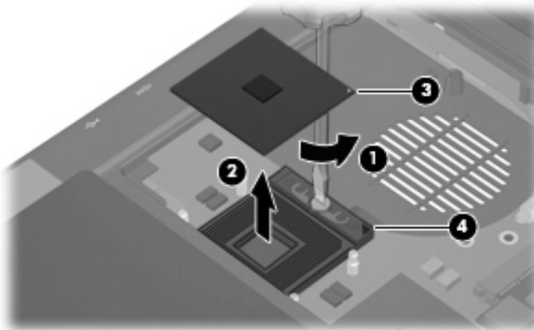
Reverse this procedure to install the processor.
