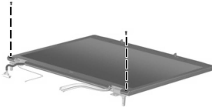
**Where used:** 2 screws that secure the display bezel bottom edge to the display enclosure
