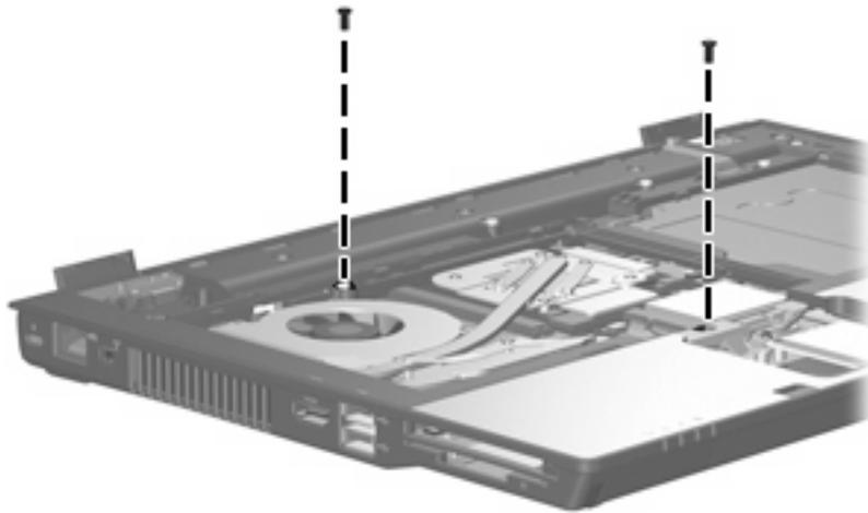
**Where used:** 2 screws that secure the top cover to the base enclosure
