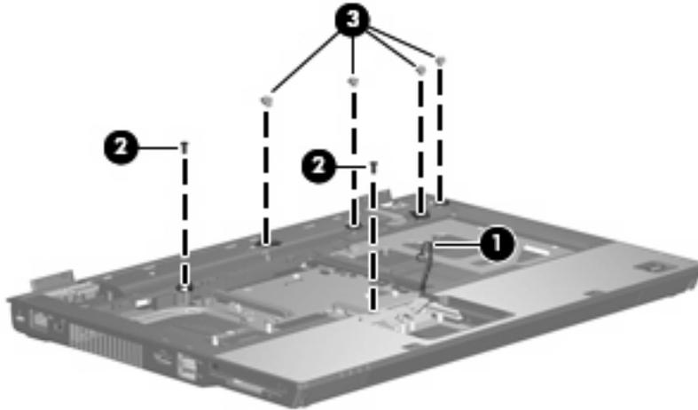
7. Lift the rear edge of the top cover **(1)** and swing it up and forward until it rests at an angle.
