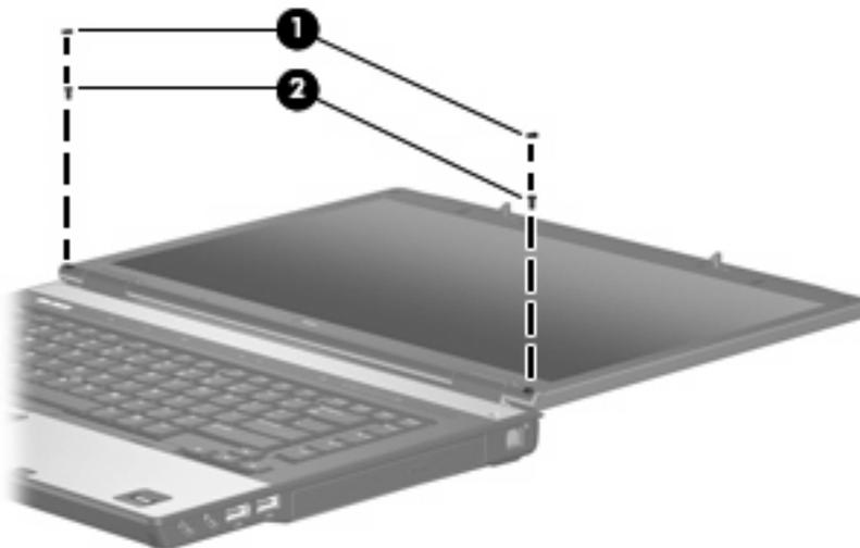
5. Flex the inside edges of the left and right sides **(1)** and the display bezel bottom edge **(2)** until the bezel disengages from the display assembly.
