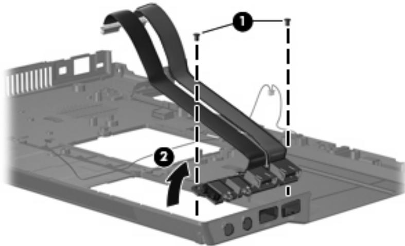
3. Remove the USB/audio board and cables from the base enclosure.
