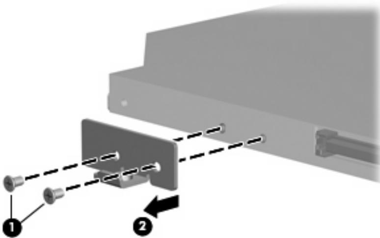
Reverse this procedure to install an optical drive.
