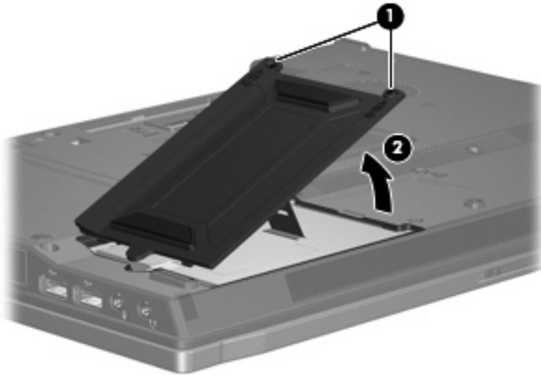
4. Loosen the Phillips PM2.5×11.0 captive screw (1) that secures the hard drive to the computer.
