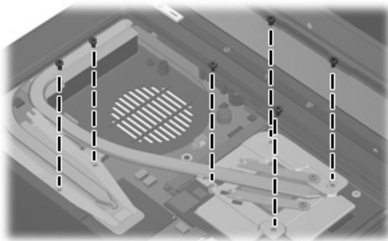
**Where used:** 6 screws that secure the heat sink to the system board
