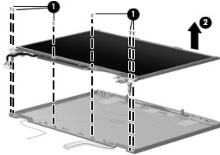
12. Remove the four Phillips PM2.0×4.0 screws **(1)** that secure each display hinge to the display panel.
