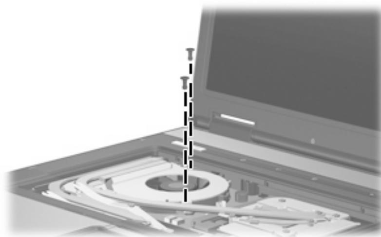
**Where used:** 2 screws that secure the fan to the base enclosure
