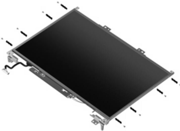
**Where used:** 8 screws that secure the display hinges to the display panel
