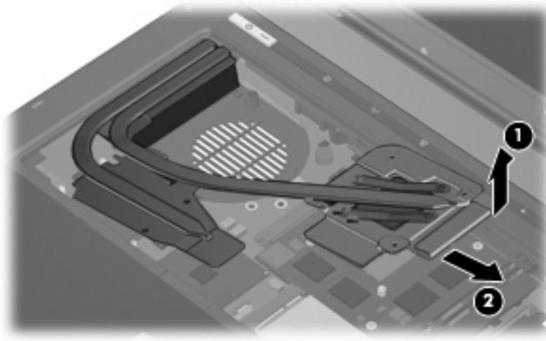
**NOTE:** The thermal material must be thoroughly cleaned from the surfaces of the heat sink **(1)** and **(3)**, the processor **(2)**, and graphics system component **(4)** each time the heat sink is removed. Thermal material is included with all heat sink and processor spare part kits.
