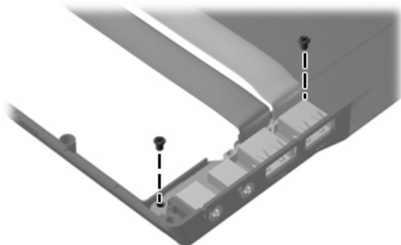
**Where used:** 2 screws that secure the USB/audio board to the base enclosure
