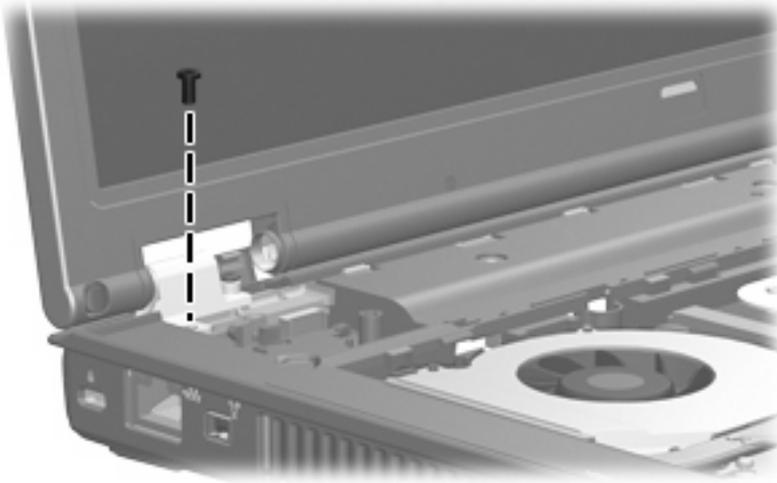
**Where used:** One screw that secures the display assembly to the computer
