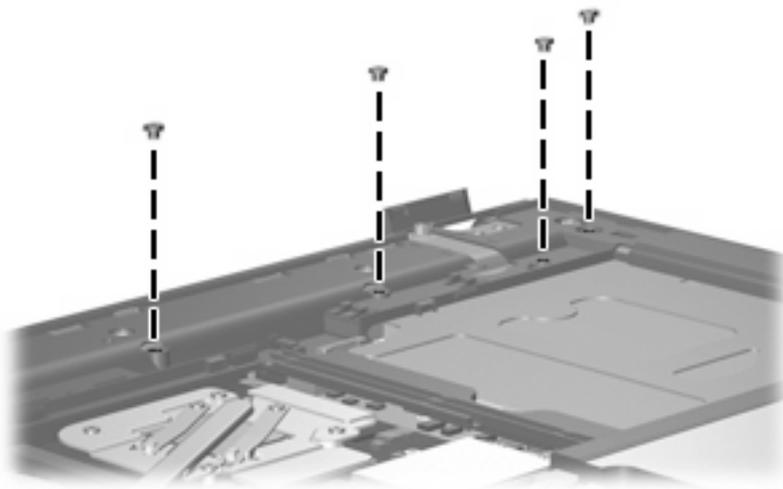
**Where used:** 4 screws that secure the top cover to the base enclosure
