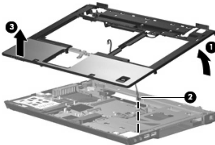
10. If it is necessary to replace the microphone, turn the top cover upside down with the front toward you.
