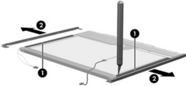
11. Remove the screws **(1)** that secure the backlight cover to the display panel.
