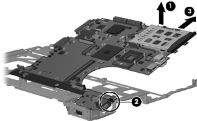
Reverse the preceding procedure to install the system board.
