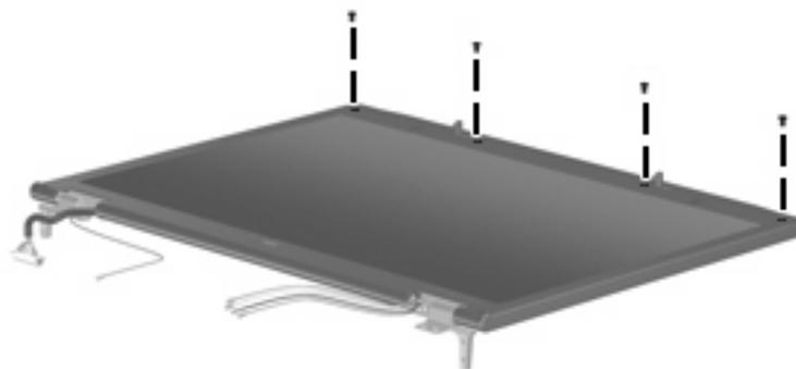
**Where used:** 4 screws that secure the display bezel top edge to the display assembly
