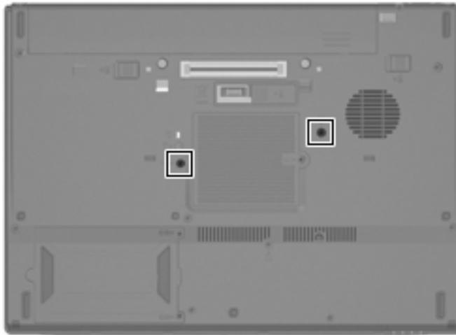
**Where used:** 2 captive screws that secure the keyboard to the computer
