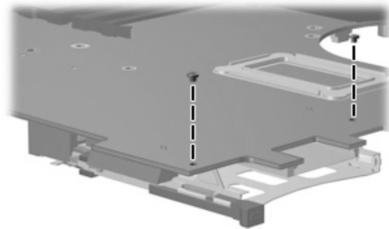
**Where used:** 2 screws that secure the PC Card assembly to the system board
