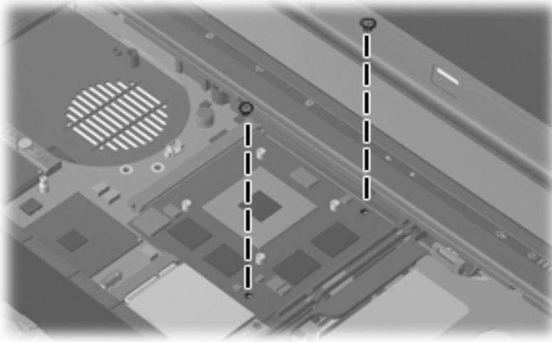
**Where used:** 2 screws that secure the graphics card to the system board
