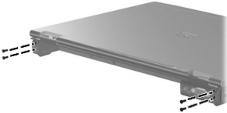
**Where used:** 4 screws that secure the display assembly to the computer
