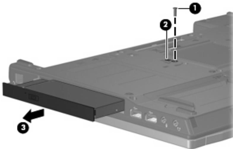
5. If it is necessary to replace the optical drive bracket, position the optical drive with the rear toward you.
