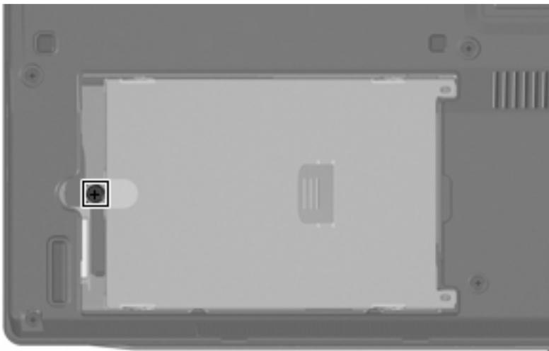
**Where used:** One screw that secures the hard drive to the computer
