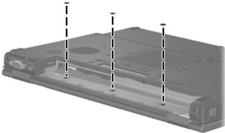
**Where used:** 3 screws that secure the switch cover to the computer
