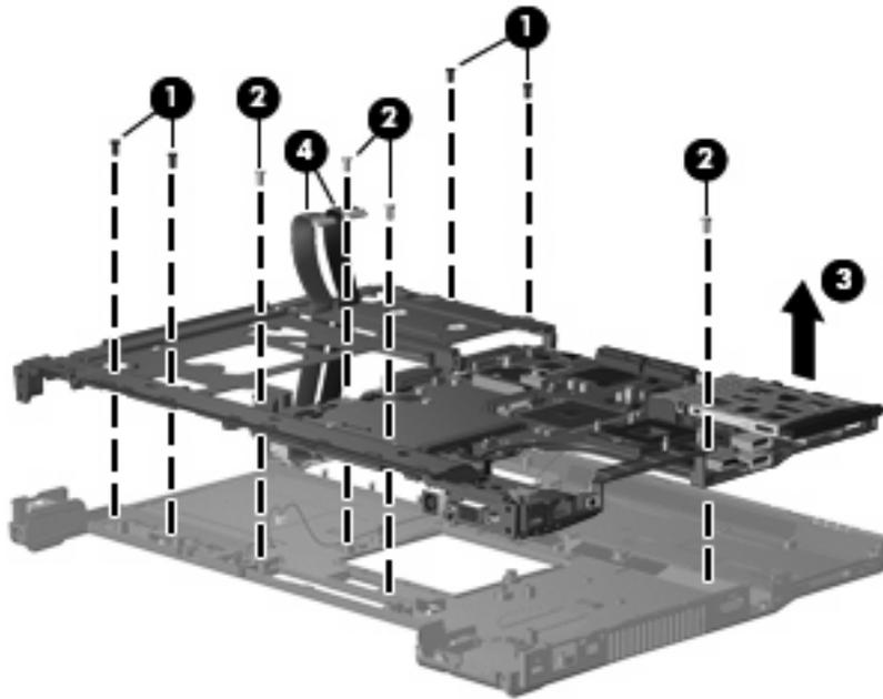
5. Remove the silver Phillips PM2.5×7.0 screw **(1)** and the two HM5.0×9.0 screw locks **(2)** that secure the system board to the system board frame.
