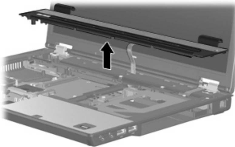
Reverse this procedure to install switch cover.
