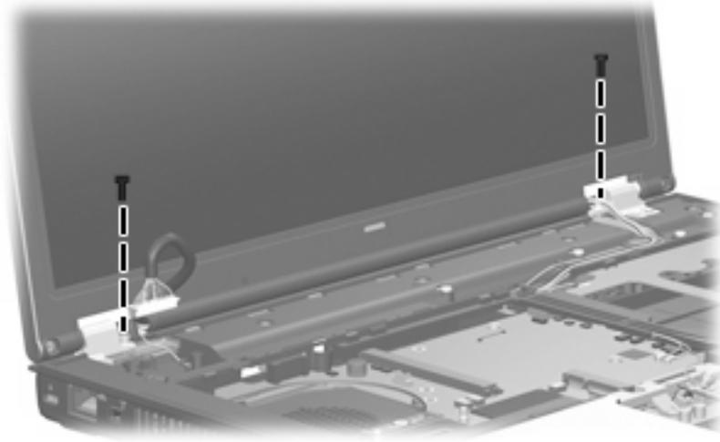
**Where used:** 2 screws that secure the display assembly to the computer
