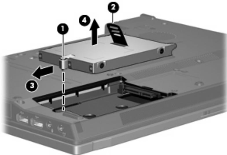
7. If it is necessary to replace the hard drive bracket, remove the two Phillips PM3.0×4.0 hard drive bracket screws (1) from each side of the hard drive.
