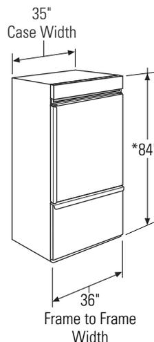
\* Shipping height. The height may be adjusted from 83-1/2" to 84-1/2" by adjusting leveling legs and wheels.
