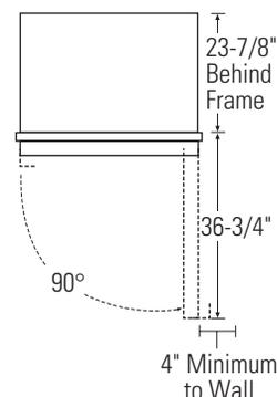
Allow 25" minimum clearance for a full 130° door swing. Allow 15" for pan removal.
