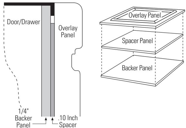
**NOTE:** Left-to-right offset is not always equal to top-to-bottom offset.
