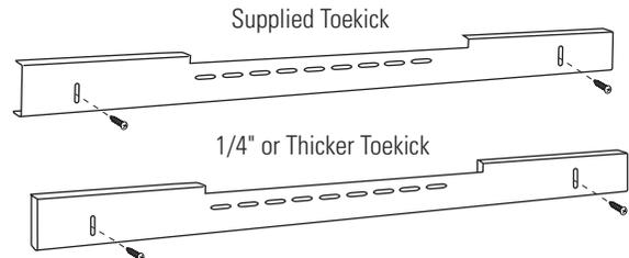
**Important:** The vented toekick must remain unobstructed for proper air circulation and refrigerator operation.
