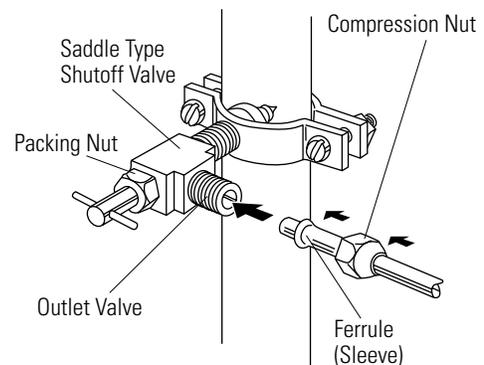
**NOTE:** Saddle type shut-off valves are included in many water supply kits. Before purchasing, make sure a saddle type valve complies with your local plumbing codes.
