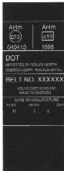
The above is a sample of the label found on all seat belts equipped with tensioners, located on the front seat belts near the lower anchorage point.
