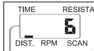
**The lower display**—The lower display will show the approximate number of calories you have burned and your pedaling speed. The display will change from one number to the next every few seconds, as shown by the indicators in the display. The display will also show your heart rate (pulse) when you use the handgrip pulse sensor or the optional chest pulse sensor.
