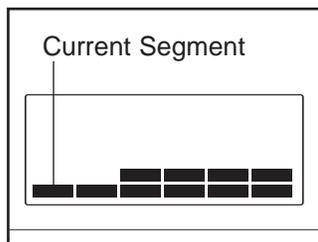
of the matrix. The target heart rate settings for the next five segments will be shown in the columns to the right. When only three seconds remain in the first segment of the program, a series of tones will sound; *all target heart rate settings will then move one column to the left.* The target heart rate setting for the second segment will then be shown in the flashing Current Segment column.
