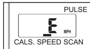
If desired, you can select a single mode for continuous display. Press the right Mode button repeatedly until the desired mode indicator is lit; make sure that the Scan indicator is not lit.
