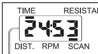
your pedaling pace, in revolutions per minute (RPM). The display will change from one number to the next every few seconds, as shown by the indicators in the display. Note: When a program is selected, the display will show the time *remaining* in the program instead of the elapsed time. Each time the resistance of the pedals changes, the display will show the resistance level.
