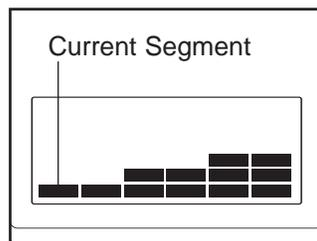
When only three seconds remain in the first segment of the program, a series of tones will sound; *all resistance settings will then move one column to the left*. The resistance setting for the second segment will then be shown in the flashing Current Segment column and the resistance of the pedals will automatically change to the resistance setting for the second segment.
