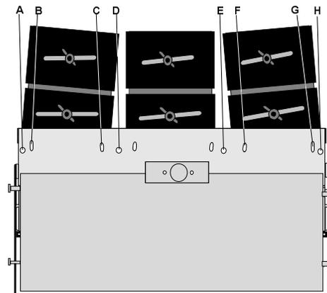
Loosen bolts E, F, G and H to pivot the blue CRT until the center of the Blue image and the center of the Green image coincide. When the angle of the blue CRT is corrected, tighten the four bolts. Press the <ENTER> key to continue with the diagonal focusing menu. Press the <EXIT> key to return to the CRT projection angle adjustment.
