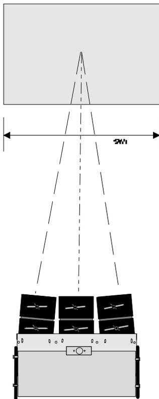
The same projection angle is misaligned for new screen width SW2. Realignment is necessary. Each screen width change requires readjustment of the projection angle.
