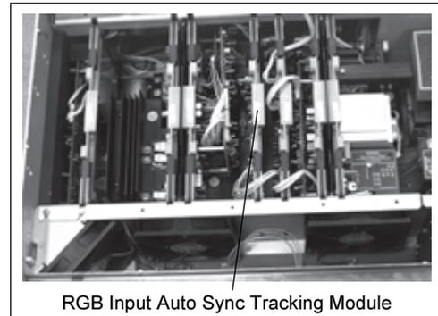
**Blue in Green Switch on the RGB Input Auto Sync Tracking Module**
