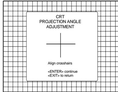
Projection angle correctly aligned for screen width SW1.
