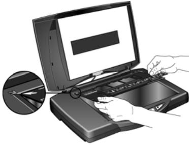
2. Follow the printed directions on the mask and place the 35mm slides horizontally into the slide holder.
