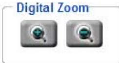
Press “+” or “-“ button to enlarge / reduce the displayed image. (max. is X10)
