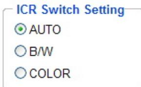
AUTO: ICR switches automatically according to the illumination.
