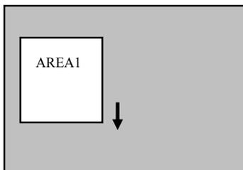
3. Increase TOP scale value by 20. AREA1 position after change is: TOP: 30, DOWN: 45, LEFT: 20 and RIGHT: 40.
