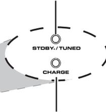
**CHARGE** indicator lights red when the speaker is turned off and rechargeable batteries are loaded
