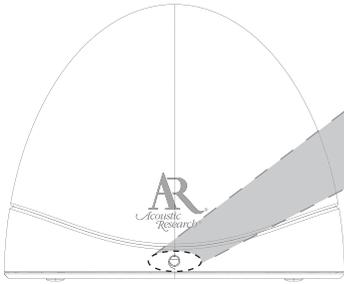
**Transmission indicator** lights blue when the audio is present and the transmitter is broadcasting
