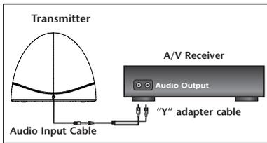
1. Connect the included "Y" adapter cable to the 3.5mm mini-plug cable coming out of the transmitter.
