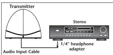
Plug the cable coming out of the transmitter into the headphone output of your stereo or the audio output jack on your computer. Use the included 1/4" headphone adapter to convert the 3.5mm plug to a 1/4" plug as needed.
