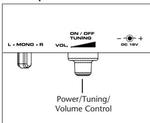
1. Press the ON/OFF/TUNING/VOL. control on the side of the speaker to turn it on. The STDBY./TUNED light on the front of the speaker illuminates red while the speaker is tuning to the transmitter. The STDBY./TUNED light turns blue when the speaker is tuned to the transmitter—you should hear sound coming from the speaker now.
