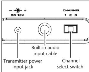
2. Set the channel select switch on the back of the transmitter to one of the transmitter's three broadcast frequencies: 1, 2 or 3. If you experience poor reception or interference, try choosing a different frequency by moving the channel select switch to another position.
