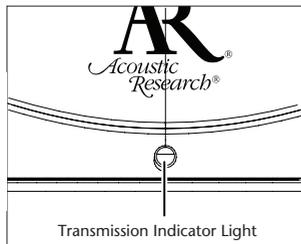
When the transmitter is receiving an audio signal and is ready, the light on its front turns blue.
