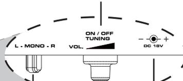
**Speaker power input jack** receives the small round end of one of the included 18V 700mA AC power adapters
