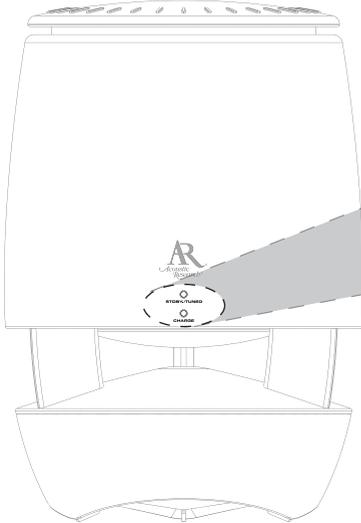
**STDBY./TUNED** indicator lights red when the speaker is first powered on; it turns blue when the speaker is tuned to the transmitter
