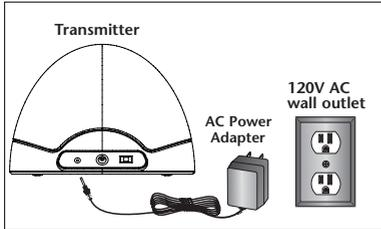
**Note:** Be sure to use the AC power adapter rated 12V DC 100 mA.
