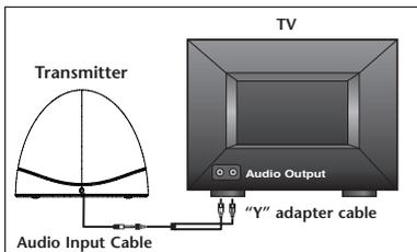
1. Connect the included "Y" adapter cable to the 3.5mm mini-plug cable coming out of the transmitter.
