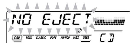
"NO EJECT" flashes on the display for about 5 seconds, and the disc is locked and cannot be ejected.
