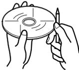
To remove these rough spots, rub the edges with a pencil or ball-point pen, etc.
