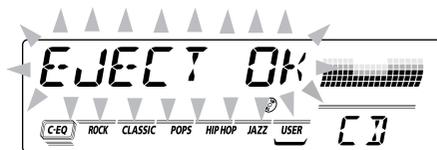
"EJECT OK" flashes on the display for about 5 seconds, and the disc is unlocked.
