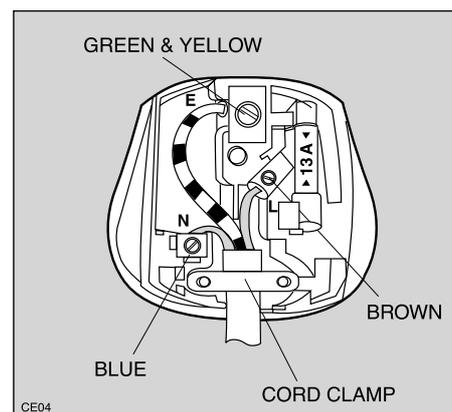
The plug must not be used if the fuse cover/carrier is lost. The cover/carrier is indicated by the coloured insert at the base of the plug.
