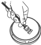
4. Position the base of the Smoke Alarm over the mounting bracket and turn. The Alarm can be positioned over the bracket every 60°. Turn the Smoke Alarm clockwise (right) until the unit is in place.
