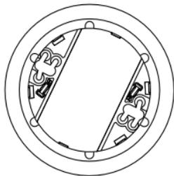
**The Mounting Bracket:** To remove the mounting bracket from the Smoke Alarm base, hold the Smoke Alarm base firmly and twist the mounting bracket off. The mounting bracket installs onto the junction box. It has a variety of screw slots to fit most boxes.
