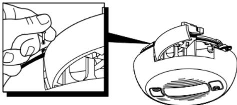
3. When you attach the Smoke Alarm to the mounting bracket, the locking pin's head will fit into a notch on the bracket.
