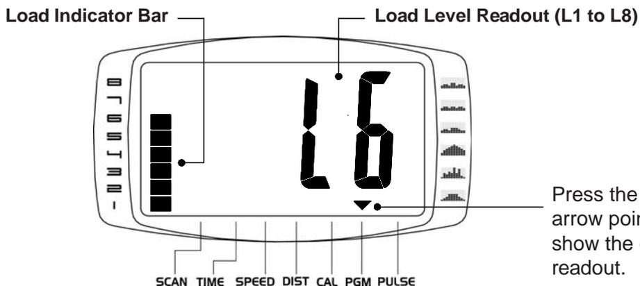
Press the **MODE** button until the arrow points to **PGM** function to show the current Load Level readout.
