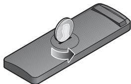
2. Remove the used battery and insert the new one (CR2032 or DL2032). Refer to page ii for battery information and safety instructions. Be sure the battery is flat side up, with the positive (+) symbol in view.
