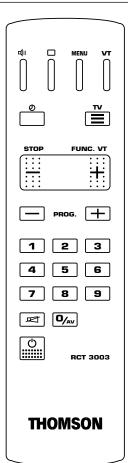
**Batteries:** Remove the lid at the back of the remote control and insert two 1,5 V batteries, TYPE LRO3 (AAA) or equivalent.
