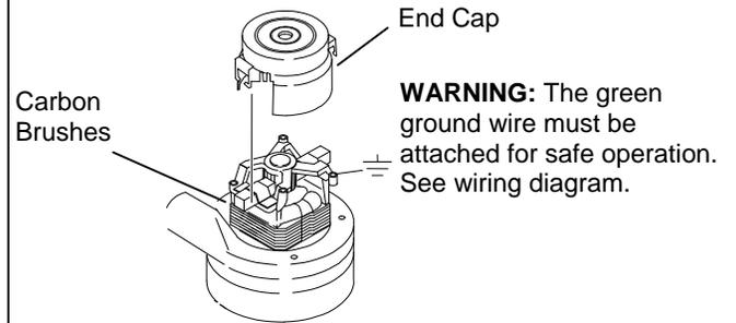
**Note:** When replacing carbon brushes loosen wire terminal **BEFORE** removing screws on bracket.
