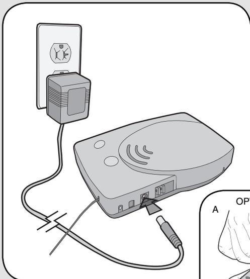
Plug in Base Station. Adhere rubber pads to bottom. A 9-Volt battery (not provided) is optional in case of power failures.
