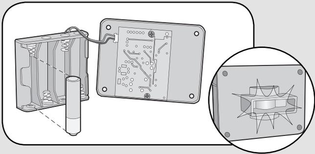
Install 4 AA Alkaline batteries (not provided). (Lithium batteries recommended for colder environments.) Test light will flash.
