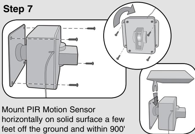
Mount PIR Motion Sensor horizontally on solid surface a few feet off the ground and within 900' of Base Station (rotate sensor to access screw holes). Unit should be able to swivel as needed. Attach sun/rain shield.
