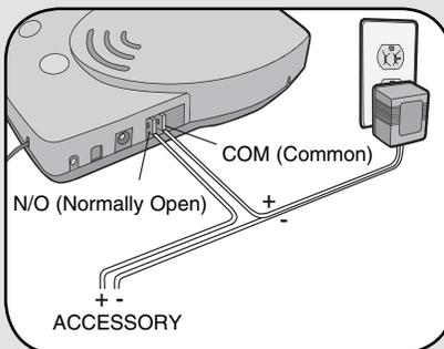
The Base Station has a relay which can activate other devices such as a low voltage doorbell, buzzer or light. The accessory device will need a separate power supply. The accessories can be purchased at any electronics store.
