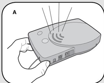
**A** Ensure Base Station and PIR Motion Sensor are in close proximity to each other. Press and release learn button on Base Station. Buzzer will sound.
