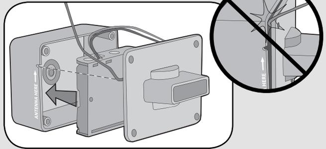
Insert battery pack facing away from circuit board and attach cover.
