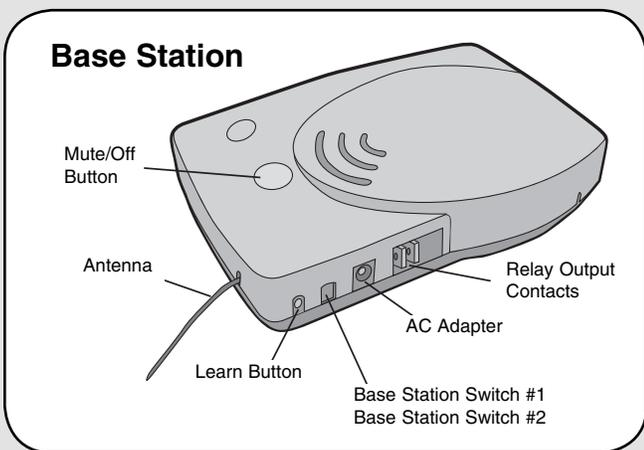
**On/Off:** To turn Base Station off hold down the Mute Button until it powers down. The Base Station can be turned on by pressing the Mute Button.
