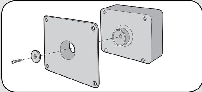
Attach PIR Motion Sensor box to mounting plate with large silver screw. Tighten screw until PIR Motion Sensor stays in place when repositioned.
