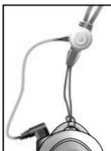
1. Loop the strap around the MP3 player's loophole and secure tightly.
