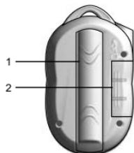
1. Battery compartment cover: Detach to install battery.
