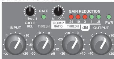
**INPUT:** Adjusts the amount of input signal to the CL151, from no signal to +20 dB.
