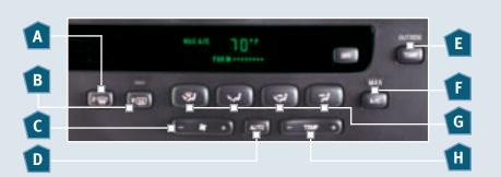
ront Window Defroster -Distributes outside air through the windshield defroster ducts. Can be used to clear ice or fog from the windshield.
