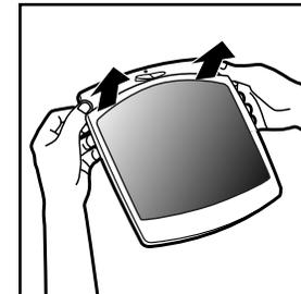
2. Remove plastic bag from the filter before installing the filter. Place the filter in the odor eliminator, fitting notched corner of filter around notched edge of odor eliminator.
