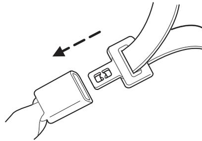
2. To unfasten, press the release button and remove the tongue from the buckle.
