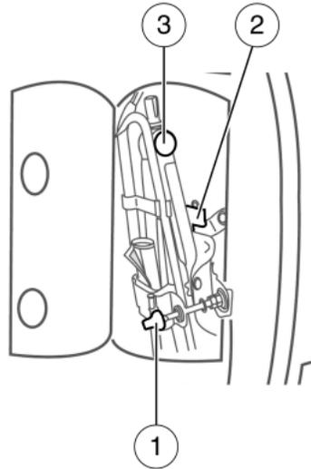
Remove the lug wrench from the jack in order to remove the spare tire from under the vehicle.
