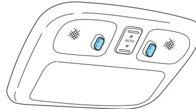
The map lamps will illuminate whenever a door is opened. After the door is shut, the lamps will remain illuminated for 25 seconds.
