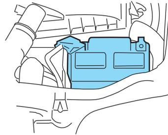
**If your battery has a cover/shield, make sure it is reinstalled after the battery has been cleaned or replaced.**
