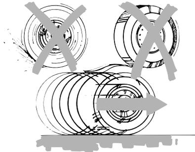
Since your vehicle has anti-lock brakes, apply the brakes steadily. Do not “pump” the brakes.
