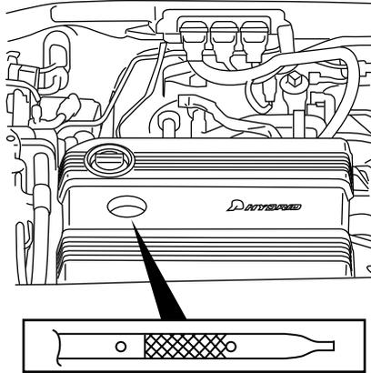
5. Locate and carefully remove the engine oil level dipstick.
