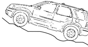
Descend a hill in the same gear you would use to climb up the hill to avoid excessive brake application and brake overheating. Do not descend in neutral; instead, disengage overdrive or manually shift to a lower gear. When descending a steep hill, avoid sudden hard braking as you could lose control. When you brake hard, the front wheels can't turn and if they aren't turning, you won't be able to steer. The front wheels have to be turning in order to steer the vehicle.
