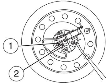
5. Use the lug wrench to remove the lug nut from the spare tire tether.
