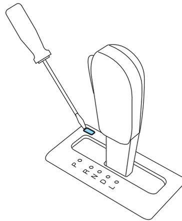
5. Remove tool and reinstall BTSI cover cap.
