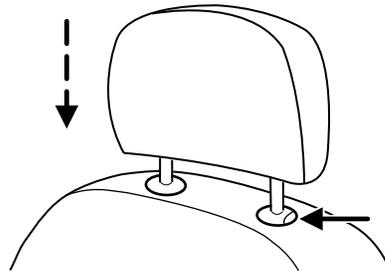
Properly adjust the head restraint so that the top of the head restraint is even with the top of your head and positioned as close as possible to the back of your head. For occupants of extremely tall stature, adjust the head restraint to its full up position.
