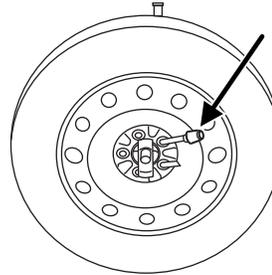
6. If not replacing the spare or flat tire to the underbody storage area, raise winch into the installed position.
