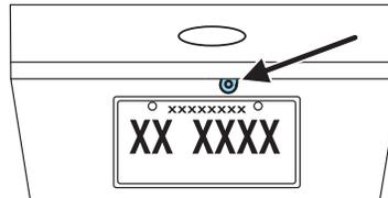
To use the camera, place the transmission in R (Reverse); an image will display on the left portion of the rearview mirror or on the navigation screen (if equipped). The area displayed on the screen may vary according to the vehicle orientation and/or road condition.
