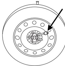
3. Lay the tire on the ground with the valve stem facing down. If your vehicle is equipped with aluminum wheels, remove the wheel ornament.
