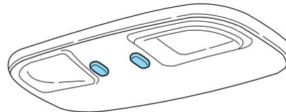
For models equipped with a moon roof, the map lamps are located on the moon roof control panel. Press the button on either side of each map lamp to illuminate the lamps. Press the button again to turn off the lamps.
