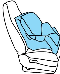
2. Pull down on the shoulder belt and then grasp the shoulder belt and lap belt together.
