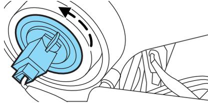
5. Disconnect the electrical connector from the bulb.
