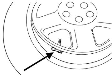
The tire pressure should be checked periodically (at least monthly) using an accurate tire gauge, refer to *Inflating your tires* in this chapter.
