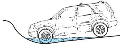
Once through water, always try the brakes. Wet brakes do not stop the vehicle as effectively as dry brakes. Drying can be improved by moving your vehicle slowly while applying light pressure on the brake pedal.
