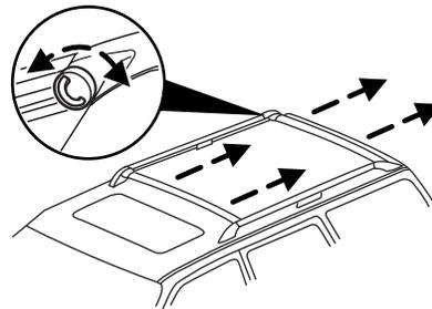
3. Use a long, flat object to depress the tongue in the endcaps on both sides of the cross-bar.
