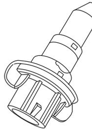
6. Connect the electrical connector on the new bulb.
