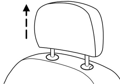
2. Press and hold the adjust/remove button, then pull up on the head restraint.
