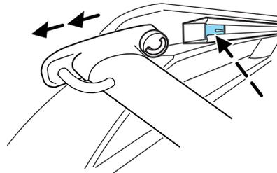
Be sure to check that the thumbwheels are tight each time load is added, or removed from the roof rack, and periodically while traveling. Always ensure the load is secure before traveling.
