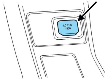
The 110V AC power point is located in the floor console in front of the gearshift.
