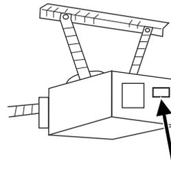
3. Return to your vehicle. Press and hold the Car2U® system button you would like to use to control the garage door. You may need to hold the button from 5–20 seconds, during which time the selected button indicator light will blink slowly. Immediately (within 1 second) release the button once the garage door moves. When the button is released, the indicator light will begin to blink rapidly until programming is complete.
