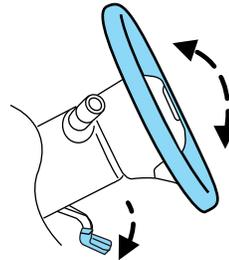
3. Push the steering column tilt lever up. This will lock the steering wheel in position.
