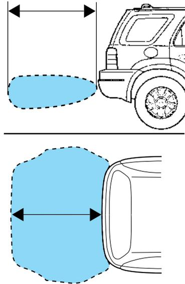
While receiving a warning the radio volume will be reduced to a predetermined level. After the warning goes away, the radio will return to the previous value. The RSS automatically turns on when the gearshift lever is placed in R (Reverse) and the ignition is on. A control in the message center allows the driver to disable the system, refer to *Message center* in the *Instrument Cluster* chapter for more information.
