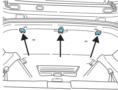
3. Clip the tether strap to the anchor as shown.
