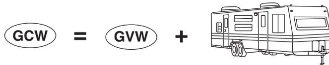
**GCW (Gross Combined Weight)** – is the weight of the loaded vehicle (GVW) plus the weight of the fully loaded trailer.
