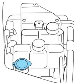
Only use a washer fluid that meets Ford specifications. Do not use any special washer fluid such as windshield water repellent type fluid or bug wash. They may cause squeaking, chatter noise, streaking and smearing. Refer to the *Maintenance product specifications and capacities* section in this chapter.
