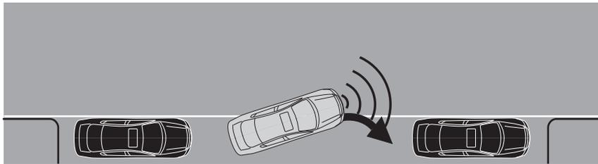
When you determine the vehicle is far enough forward or a solid tone from forward sensing system (if equipped) is heard, bring the vehicle to a complete stop and move the gearshift to R (Reverse). The message center may display BACK UP SLOWLY USE CAUTION followed by a chime. The system may offer subsequent backward and forward maneuvers before proceeding to the finish phase.
