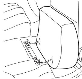
Attach the safety belt web snap button to the quarter trim panel snap button. This will ensure that safety belt does not get caught by staying out of the seat back folding path.
