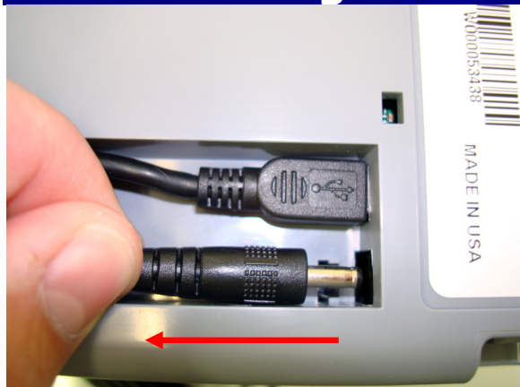
Fig. 13 The correct way to remove a cable.
