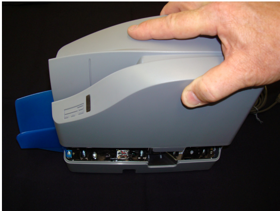
Fig. 12 Replace the center cover by setting it back on the unit vertically.
