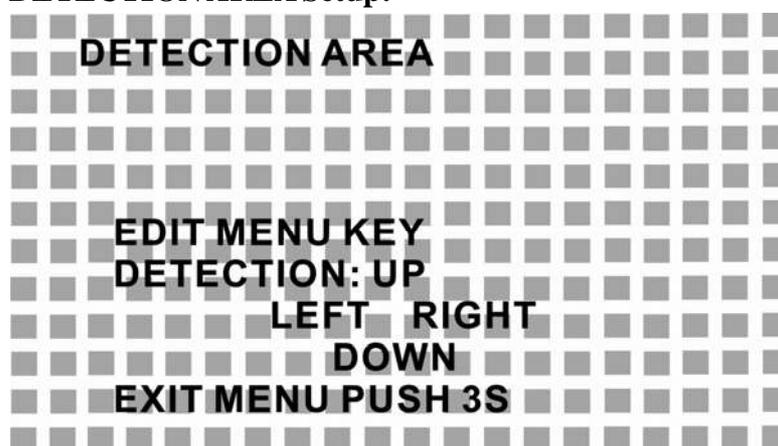
Detection Block Setup: Press MENU button to enable or disable a single cell configuration setting Use up and down keys to move around or to end the setting mode. Press MENU button for 3 seconds to leave the setting page.
