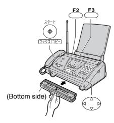
Insert the hand scanner in the main unit or press
