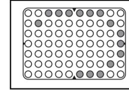
**DISTANCE/LAPS display**—This display shows the distance that the walking belt has moved and the number of 1/4-mile laps you have completed. The display will alternate between one number and the other every seven seconds; the indicator will light when the number of laps is shown.
