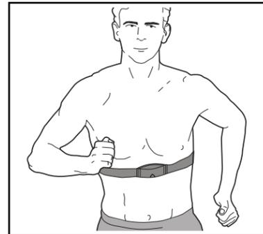
Pull the sensor unit away from your body a few inches and locate the two electrode areas on the inner side. The electrode areas are the areas covered by shallow ridges. Using saline solution such as saliva or contact lens solution, wet both electrode areas. Return the sensor unit to a position against your chest.
