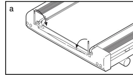
b. **If the walking belt has shifted to the right**, first remove the key and **UNPLUG THE POWER CORD**. Using the allen wrench, turn the left rear roller adjustment bolt counterclockwise, and the right bolt clockwise, 1/4 of a turn each. Be careful not to overtighten the walking belt. Plug in the power cord, insert the key and run the treadmill for a few minutes. Repeat until the walking belt is centered.
