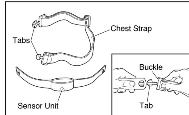
Next, wrap the heart rate monitor around your chest and attach the other end of the chest strap to the sensor unit. Adjust the length of the chest strap, if necessary. The heart rate monitor should be under your clothing, tight against your skin, and as high under the pectoral muscles or breasts as is comfortable. Make sure that the logo on the sensor unit is facing forward and is right-side-up.
