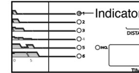
Note: The graphs on the left side of the console show how the speed or incline of the treadmill will change during the programs. During program 4, for example, the graph shows that the incline will gradually increase during the first half of the program and then gradually decrease during the last half.
