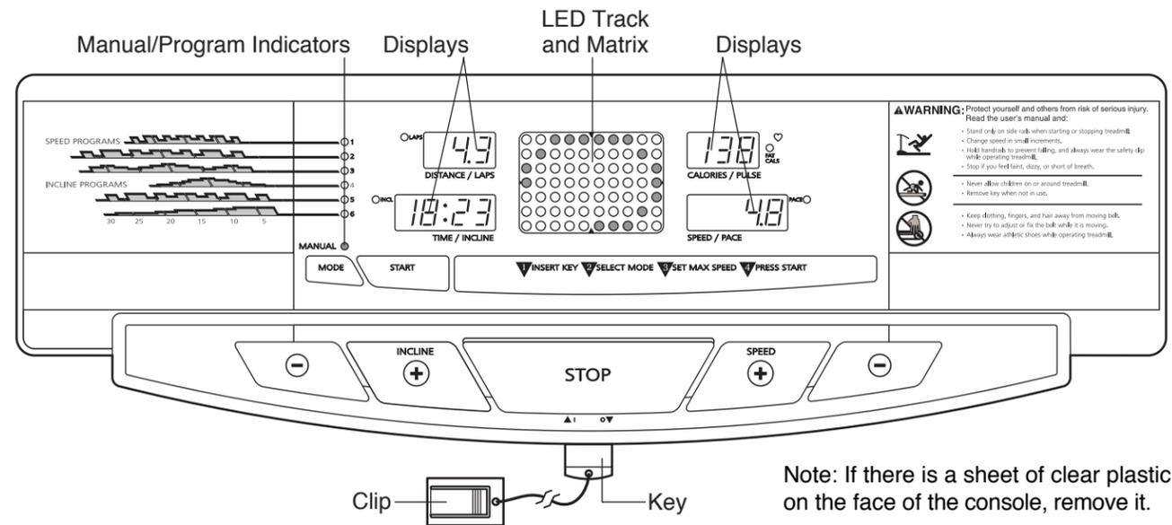
Note: If there is a sheet of clear plastic on the face of the console, remove it.
