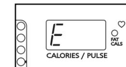
**CALORIES/PULSE display**—This display shows the approximate numbers of calories and fat calories you have burned (see FAT BURNING on page 15). Every seven seconds, the display will change from one number to the other; the indicator will light when the number of fat calories is shown. This display will also show your heart rate when the heart rate monitor is worn; the heart-shaped indicator will light when your heart rate is shown.
