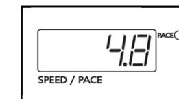
Note: The console can display distance, speed, and pace in either miles or kilometers. To see which unit of measurement is selected, hold down the STOP button while inserting the key into the console. An “E,” for english miles, or an “M,” for metric kilometers, will appear in the CALORIES/PULSE display. If you want to change the unit of measurement, press the SPEED  $\Delta$  button. Then, remove and reinsert the key.
