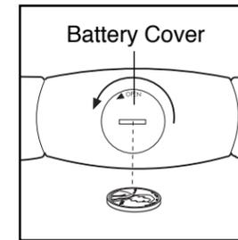
Remove the old battery from the sensor unit. Insert a new **CR 2032 battery**, making sure that the writing is on top. In addition, make sure that the rubber gasket is in place in the sensor unit. Replace the battery cover and turn it to the closed position.
