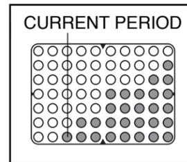
When only three seconds remain in the first period of the program, both the CURRENT PERIOD column and the column to the right will flash and three tones will sound. All speed or incline settings will then move one column to the left. The setting for the second period will then be shown in the CURRENT PERIOD column and the speed or incline of the treadmill will automatically adjust to the second setting.
