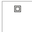
This symbol indicates that this product incorporates double insulation between hazardous mains voltage and user accessible parts. When servicing, use only identical replacement parts.
