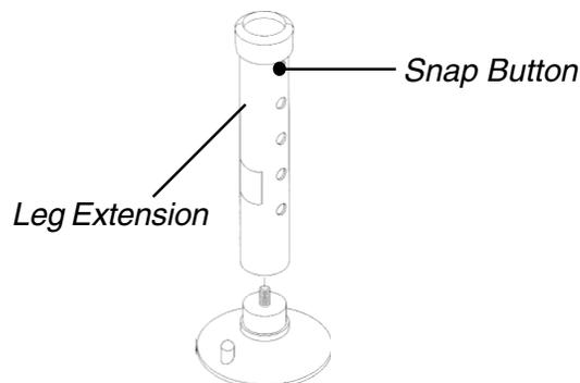
FIGURE 2 - REMOVING THE EXISTIING LEG EXTENSIONS
