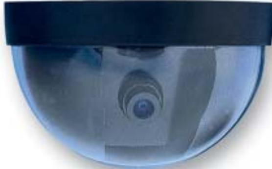
Our 1/4" color CCD dome camera with smoked housing can be mounted on the ceiling and offers unobtrusive surveillance with its' black housing. It can be rotated a full 360 degrees and tilted +/- 90 degrees for maximum viewing selection. It features 1.0 lux sensitivity with 420 line resolution and a 3.6mm wide angle lens with built-in electronic shutter. A 12V DC power supply is included.
