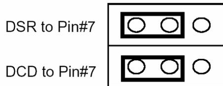
**Figure 7: Jumper Block Pin-out**
