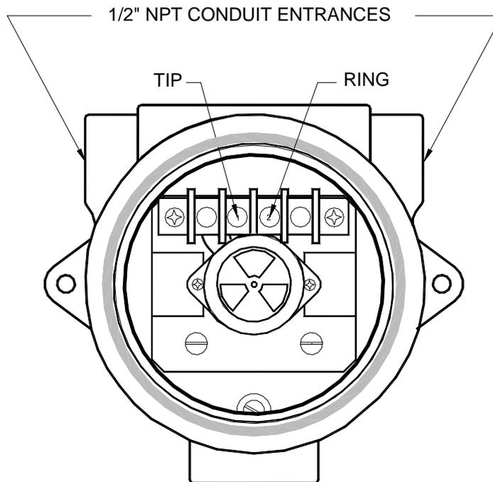
**Figure 2 - Electrical Connections**
