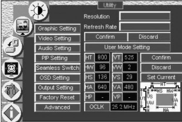
Figure 40: Output Setting User Mode Setting Utility Screen
