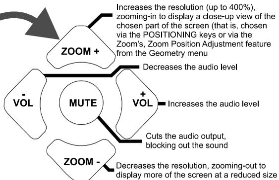
*Figure 16: Infra-Red Remote Control Transmitter*
