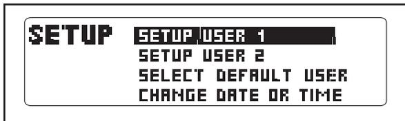
Next, highlight the SETUP USER 1 or SETUP USER 2 option and press the Enter button. The user information menu will then appear in the display.
