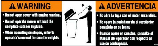
Permanently attached to grass collection system cover. ALWAYS use caution operating on hills. Counterweights are not necessary with the rear wheel motor supports properly mounted in the rearmost position. Optional deck counterweights are available to help prevent step-cutting.
