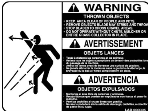
Located on blower, All components of the grass collection system must be in place during operation. If any component is missing, it must be replaced before continuing operation. Either the blower or discharge chute should be in use at all times. Failure to comply could result in serious injury or death.
