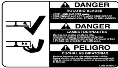
Located on blower, Always use caution with movable parts. Serious injury can result from working on your grass collection system with the mower in operation. Always turn off machine and remove key before dislodging any jammed objects. Also be cautious of spinning components after an obstruction has been removed from the system.
