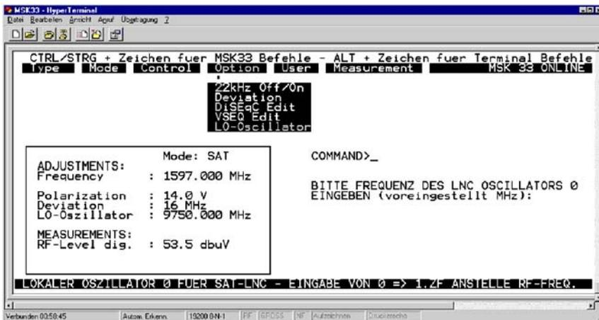
Example: Entry of the LNB oscillator frequency
