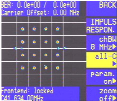
Hierarchy = 1 means, that the signal is hierarchically modulated. Two transport streams are simultaneously transmitted, one has higher priority in QPSK.
