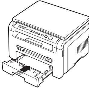
**NOTE:** After you load paper, you need to set up your machine for the paper type and size you loaded. See page 3.6 for copying, or the **Software Section** for PC-printing. The settings made from the printer driver override the settings on the control panel.
