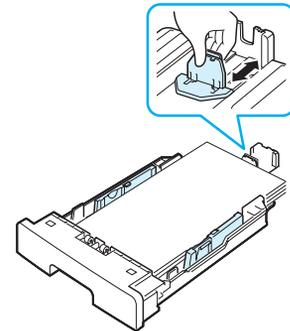
For paper smaller than Letter size, adjust the front paper length guide so that it lightly touches the paper stack.
