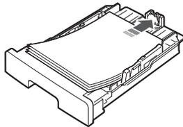
You can load letterhead paper with the design side face down. The top edge of the sheet with the logo should be placed at the front of the paper input tray.
