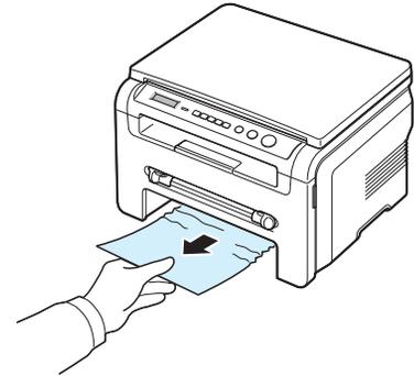
If there is any resistance and the paper does not move when you pull, or if you cannot see the paper in this area, check the fuser area around the toner cartridge. See page 9.2.
