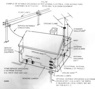
d Use jumper wire not smaller than No. 6 AWG (13.3 mm²) copper, or the equivalent, when a separate antenna-grounding electrode is used. See NEC Section 810-21 (j).
